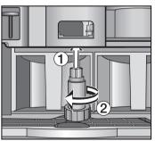
Insert the tool for removing the perforator up into the unit, ①. Turn it to the left, ②, to loosen and remove the perforator.
